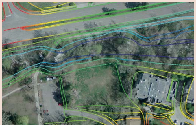
Figure 2. Ortho with mass points and breaklines superimposed.
