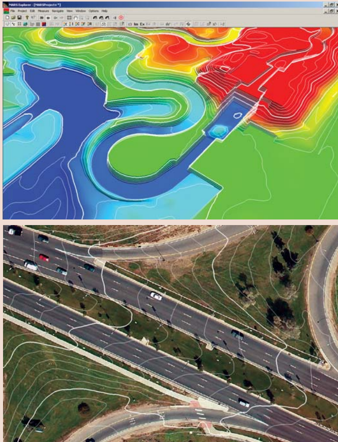
Figure 5. Illustrates; shaded relief with contours in 3D (ul), 3D lidar intensity (ur), ortho with real-time contour generation (ll), and 3D gradient color cycles (lr).
