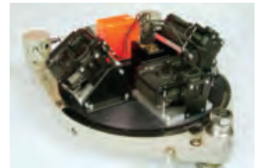
Figure 3. The DLR-3k three-camera system makes use of a fan of three Canon EOS small-format digital cameras with one firing vertically and two obliquely to provide wide cross-track coverage.
