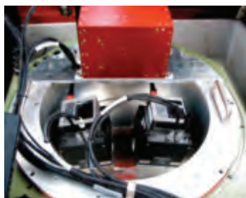
Figure 2. The IGI Dual-DigiCAM system featuring twin oblique pointing digital cameras mounted on a gyro-stabilized platform.
