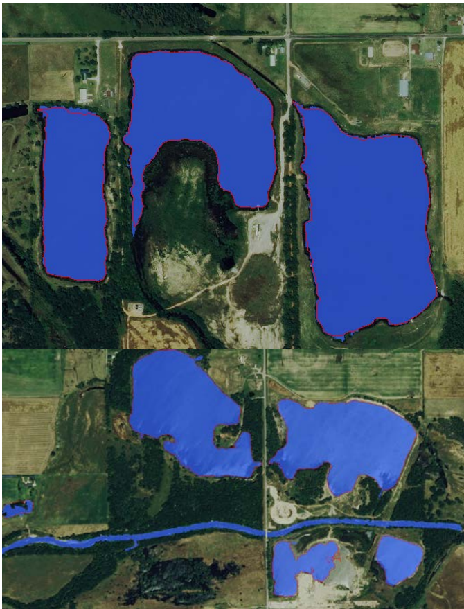
Fig. 08. Seven main water-bodies in Oklahoma dataset. Manually detected border (Red lines) and Algorithm detected water-body (Blue semi-transparent polygon).
