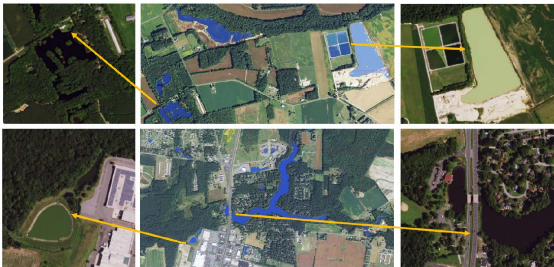
Fig.11. Detected water-body (Blue polygons) overlaid on satellite image are shown for a few small water-bodies
