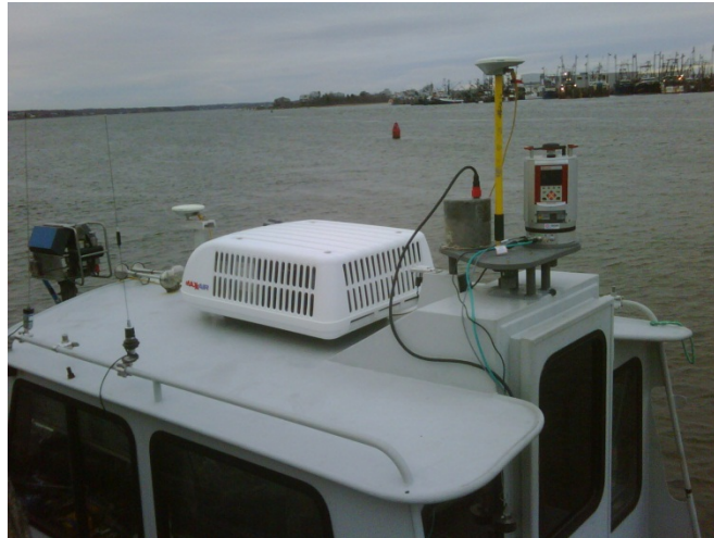
Figure 1. Mobile VZ-400 System, mounted next to the IMU.
