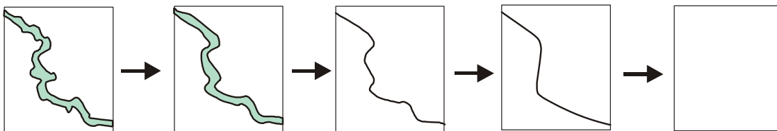
Figure 2. The generalization lifecycle of river feature, including polygon simplification, collapse, line simplification, and elimination.
