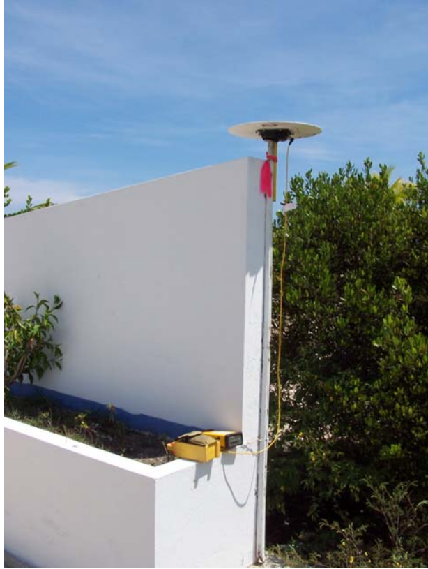
Figure 5. Photo Identifiable Control Point.
