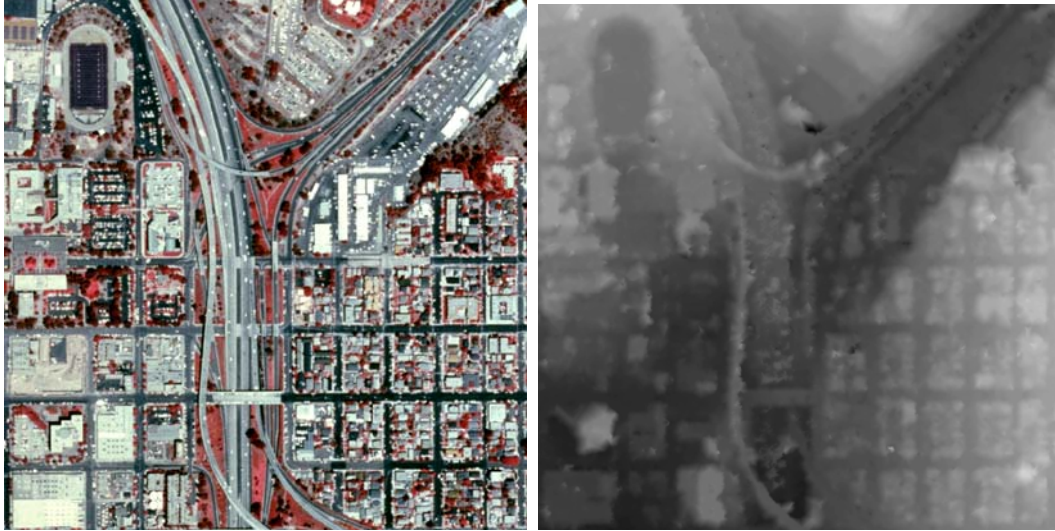
Figure 6. CIR and DSM of the Ikonos stereo test scene extend of the subset: about 900 m * 900 m, location San Diego, CA
