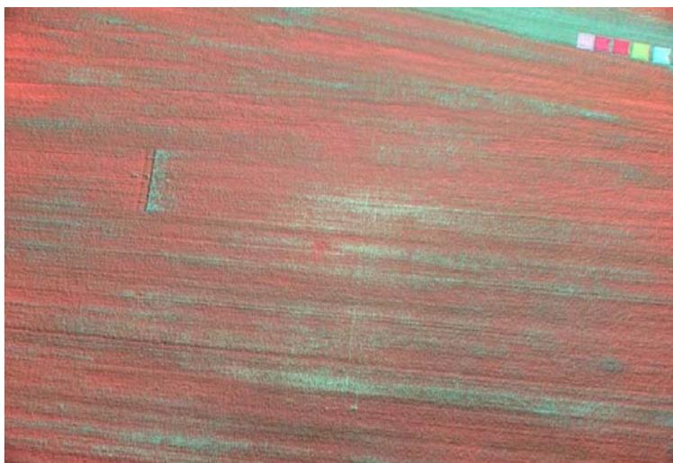
**Figure 4.** A near-infrared, green and blue digital image obtained from a small UAV flying at an altitude of 400 feet (120 m) above ground level. The near-infrared band is displayed as red. The two lines running from top to bottom in the center of the image are footpaths where the wheat was trampled slightly on the way to a sample plot. The squares along the top are colored tarpaulins used to calibrate GNDVI from digital numbers to reflectances.
