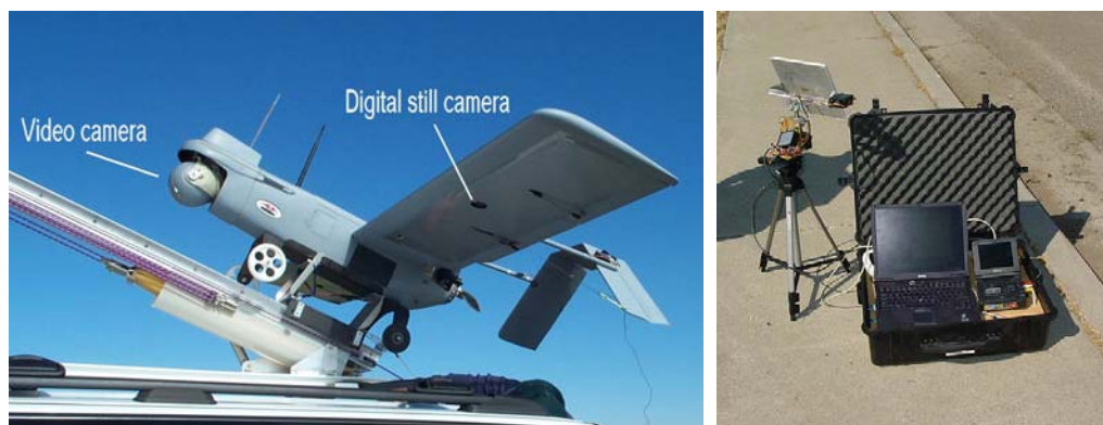
Figure 1. BAT 3 UAV on the catapult on top of the launch vehicle. The video camera is housed in a 3-axis gimbal in the nose, and the digital still camera is mounted in the left wing (left). Ground station with laptop and video deck used for live video downlink, and telemetry antenna (right).
