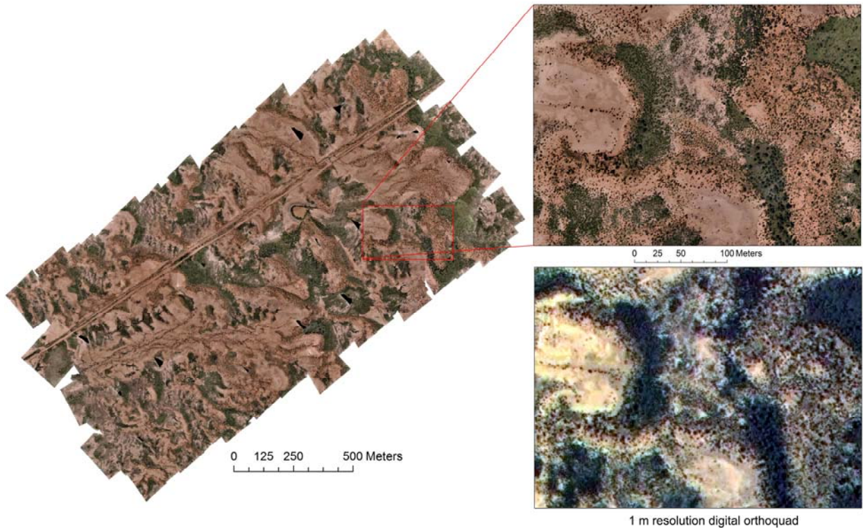
Figure 3. Orthorectified mosaic of 257 UAV images at the Jornada Experimental Range in southern New Mexico (left) with enlarged portion of red rectangle (top right), and comparison with 1 m resolution digital orthoquad image (bottom right).
