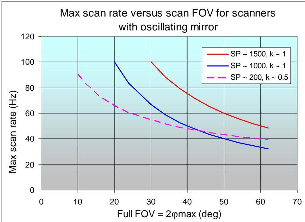
**Figure 4.** Maximum scan rate (scan frequency) versus maximum scan angle (maximum scan FOV) for oscillating mirror scanners. Dashed line represents sinusoidal scanner; solid lines represent sawtooth scanner with different scan products.
