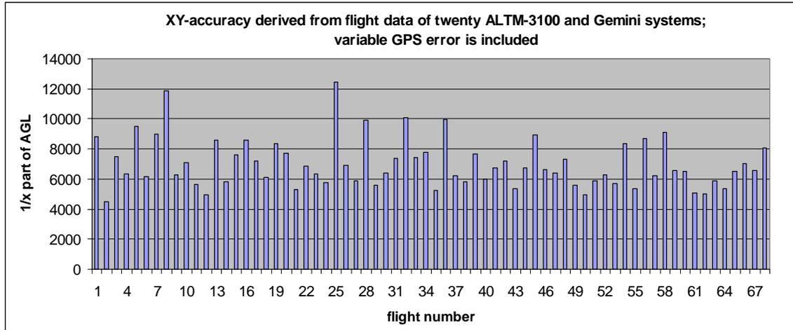
**Figure 6.** XY accuracy derived from the flight data of twenty ALTM 3100 systems at different flying altitudes, variable GPS error included.
