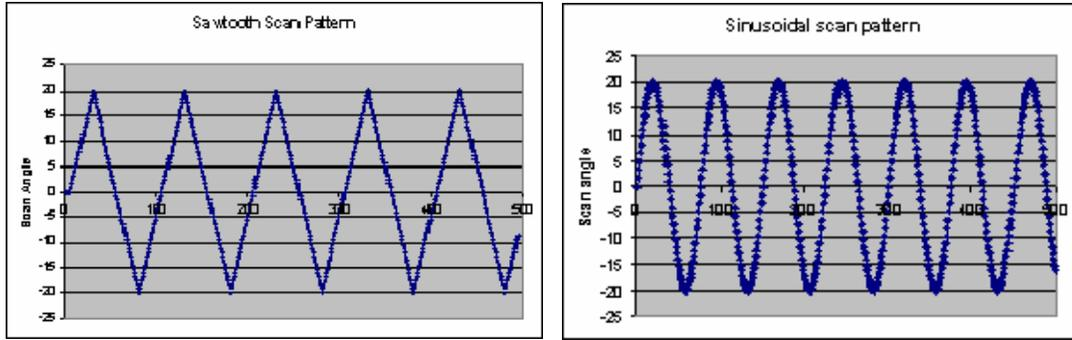
**Figure 3.** Sawtooth and sinusoidal scan patterns from an oscillating mirror scanner.
