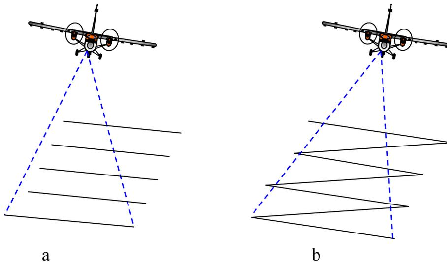
**Figure 2.** Scan pattern from constant velocity rotating polygon mirror (a), and oscillating mirror (b).
