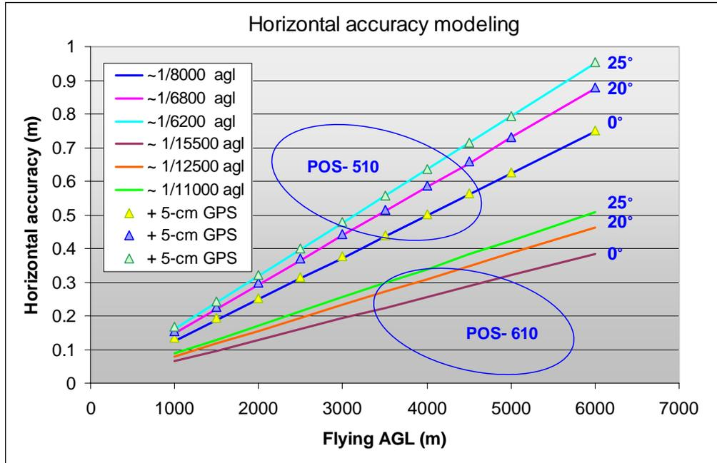
**Figure 5.** Theoretically achievable horizontal accuracy in an airborne lidar system equipped either with POS-510 or POS-610 (or equivalents) under assumptions specified above. All solid lines represent modeling results for zero GPS error; dotted lines represent the corresponding results, while a 5 cm GPS error was included.
