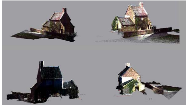
Figure 6. The 3D model of Cooks' cottage from TLS data.
