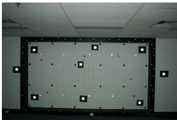
Figure 3. The calibration wall comprised of retro-reflective targets.
