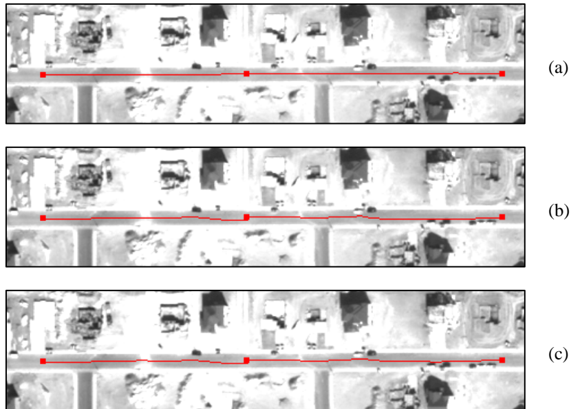
Figure 3. Road tracking results on QuickBird test site 2 using different similarity metrics: (a) mutual information, (b) SSD, and (c) cross-correlation.
