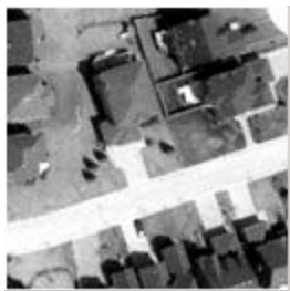
Figure 1b. Sub-ortho image after removing rotation error
