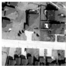
Figure 1a. Sub-ortho image with a rotation error
