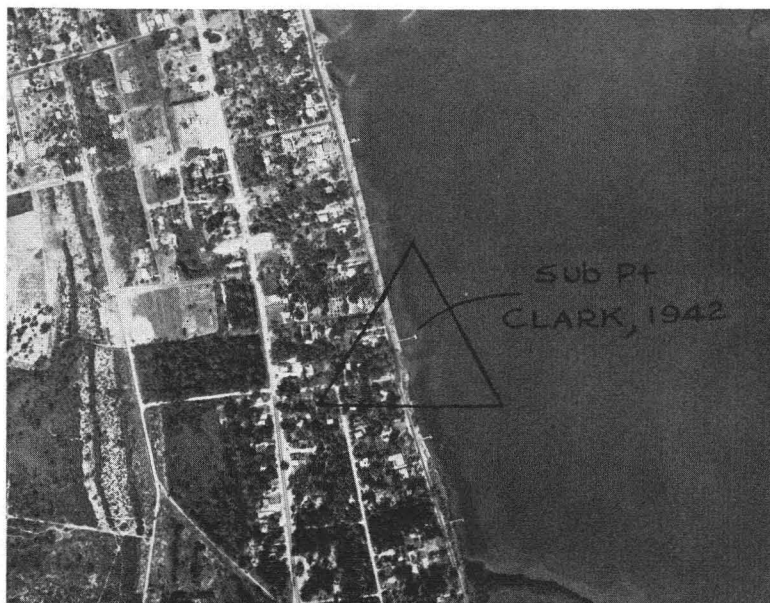
FIG. 1. Part of an aerial photograph illustrating the identification of substitute horizontal control station.
