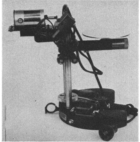
FIG. 8. Motorized Multiplex Table. A small motor driving the crown gear takes power from the regular tracing table source and is controlled by two switches at the left hand side of the table base. Photograph courtesy of United States Navy Hydrographic Office.
