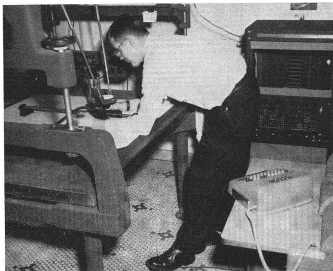
FIG. 17. Electronic Recording of Cross Sections. Center line off-set and elevation readings from the plotting table are transmitted electronically through a demodulator to the digitizing console in the upper right. The readings are then fed to the IBM Summary Punch and punched on cards together with the identification which the operator records by means of the key punch. Photograph courtesy of Ohio Highway Department.
