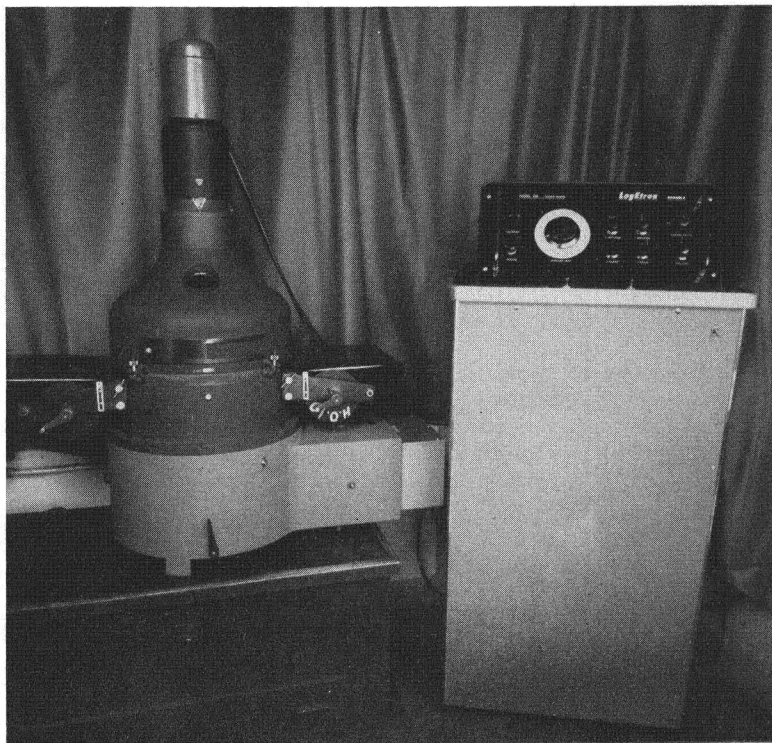
FIG. 7. Log Etronic Console Diapositive Printer. This unit is adaptable to any type of diapositive printer for Multiplex, ER-55, or Kelsh type diapositives. Photograph courtesy of United States Navy Hydrographic Office.
