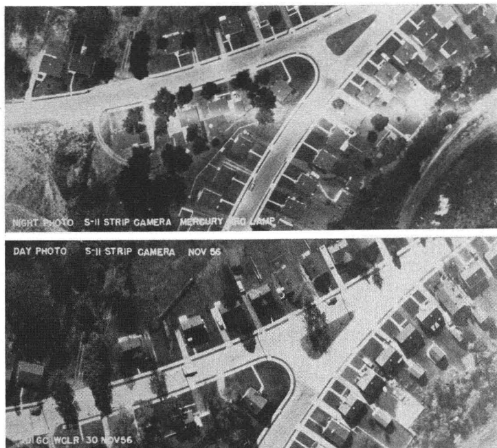
FIG. 3. Example of Night Photography Obtained with Strip Camera. The lower photograph illustrates normal daytime photography with the Strip Camera. The upper photograph shows the same area photographed at night using the high intensity mercury lamp which illuminates a very narrow strip directly underneath the aircraft. Photograph courtesy of Wright Air Development Center.
