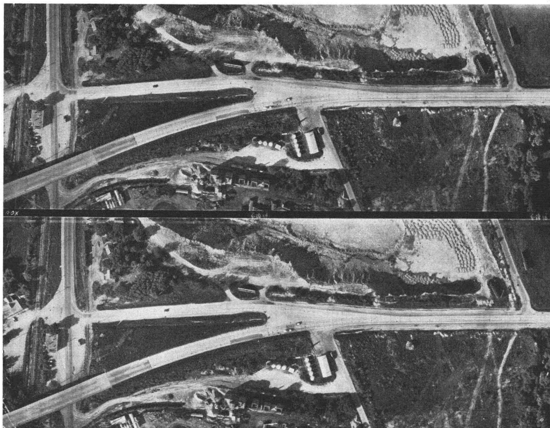
FIG. 1. Example of Sonne Strip Photography. The resolution and detail obtainable with this type of photography is apparent in this sample. Photograph courtesy of Chicago Aerial Industries, Inc.
