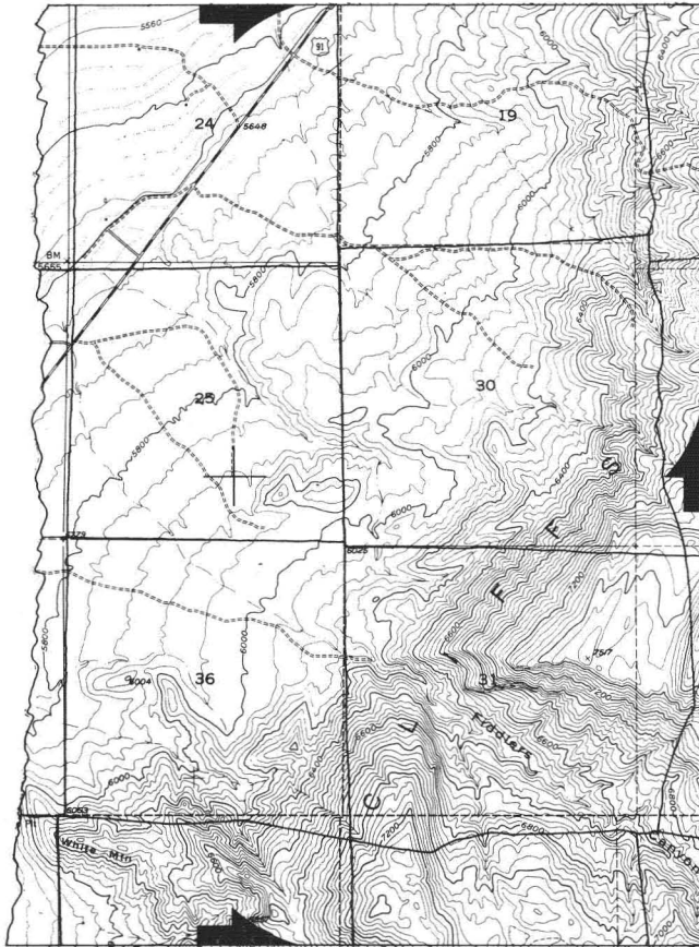
FIG. 2. Construction on northeast portion of U. S. Geological Survey topographic map of Cedar City, Utah, quadrangle (1950), showing portion of skeletal "aerial vertical photograph" taken with 6" lens from an altitude of about 12,000 feet above valley at left. Irregular graticule shows effects of relief displacement on section lines which cross rough topography at right and gently sloping piedmont plain at left. Common scale datum of map and "photograph" lies at approximately the same elevation as the base of the steep cliffs.
