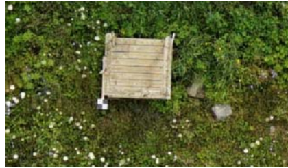
Figure 4. Photo identifiable metal checkered target affixed to wooden structure
