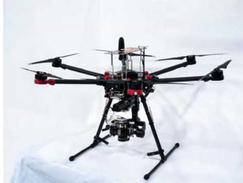
Figure 2. DJI M600 UAS with the APX-15 EI UAV and a Sony a7R camera on Ronin Gimballed Mount
