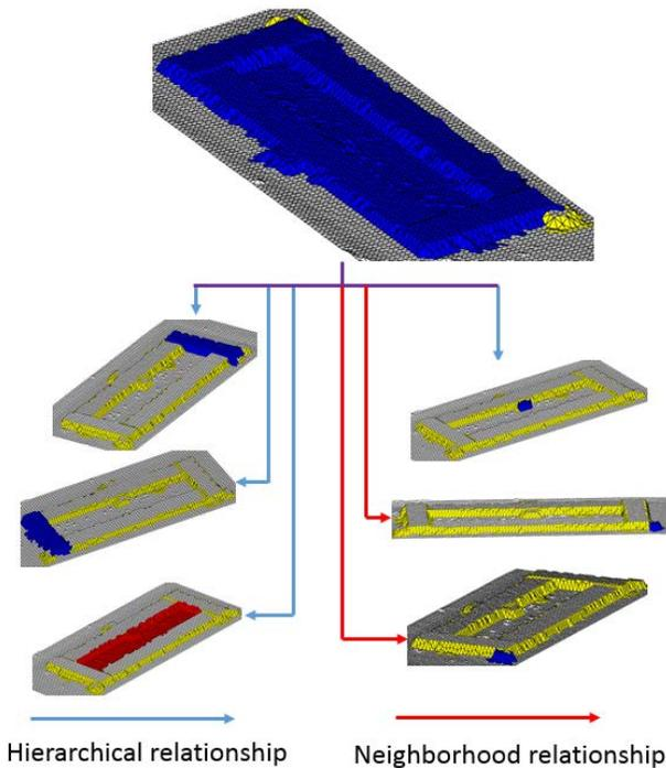
Figure 6 Hierarchical decomposition of the complex building. Blue segments represent convex structure whereas red segments represent concave structure
