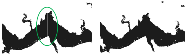
Fig. 5. The thin line in batch boundary if a waterbody is extended in two batches is shown in left figure. In right figure, the merged waterbody is shown after the removal of the thin line.
