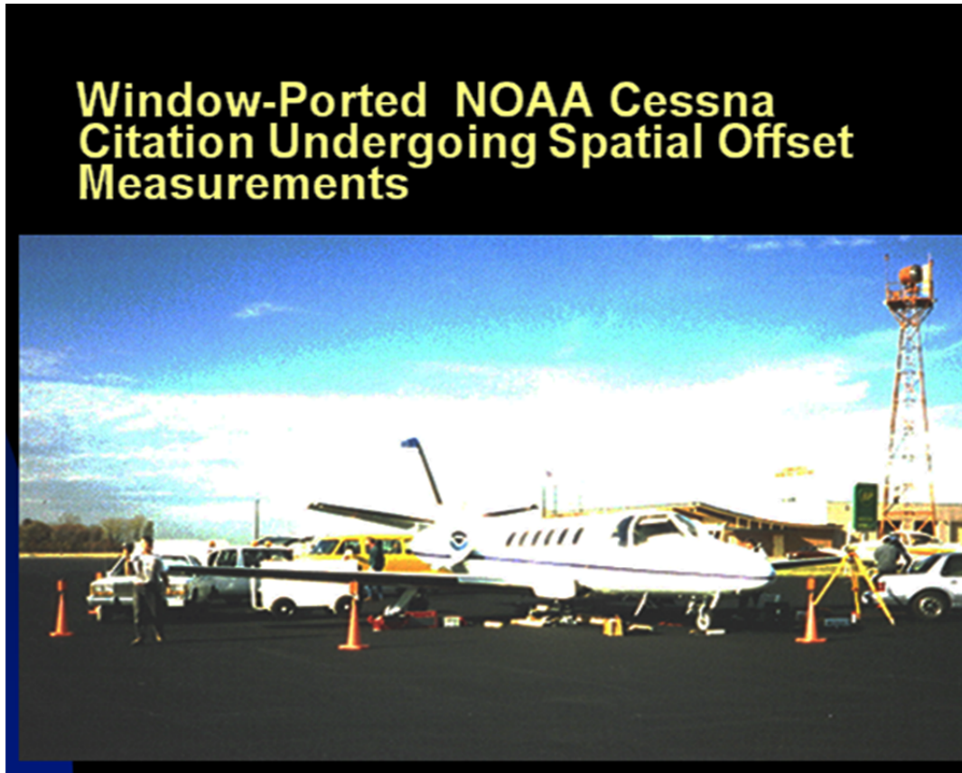
Figure 2G. NOAA Window-Ported (Pressurized) Cessna Citation Stabilized for Spatial Offset Measurements, to Phase Center to Entrance Node.
