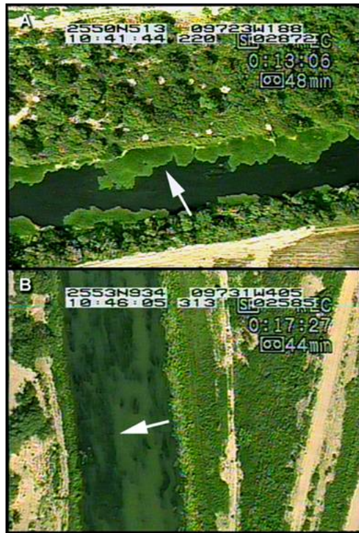
Figure 1. Aerial normal color video images of infestations of waterhyacinth (A) and hydrilla (B) in the Rio Grande River near Brownsville, Texas. The arrows point to waterhyacinth and hydrilla in each respective image. The imagery was obtained on September 19, 2002 at an altitude above ground level of approximately 600 m and had an original pixel size of approximately 0.70-m.
