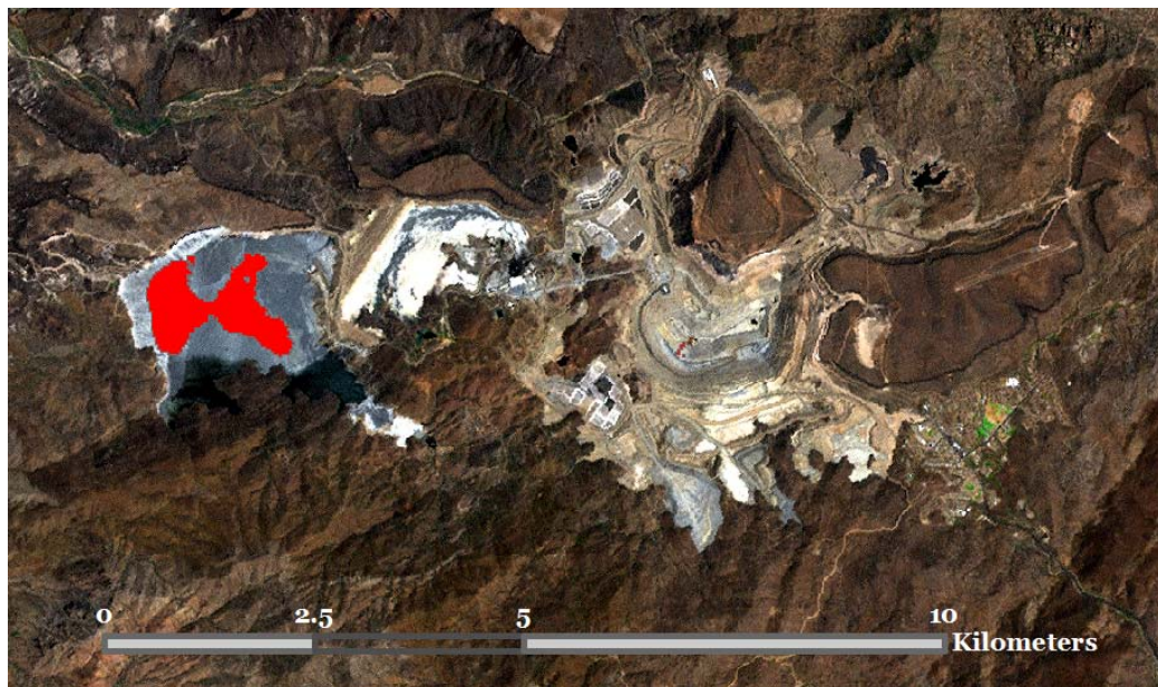
Figure 5. A 2000 Landsat 7 ETM+ scene, RGB-321, showing the Bagdad Copper Mine. The red polygon represents the results of the NDTI-Aggregate density filter, identifying the Lower Mammoth tailings impoundment.
