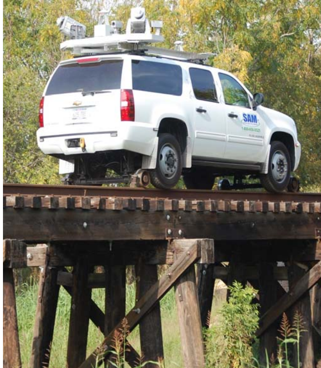
Figure 2. The Lynx Mobile Mapper on a Chevrolet Suburban adapted for hyrail operation. (Image courtesy of SAM Inc.)
