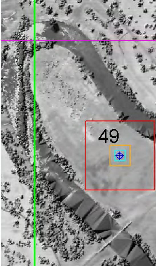
*Figure 12: Checkpoint located in a flat open area with 3 different sized areas (900 in cyan, 3,600 in orange and 40,000 square meter shown in red) surrounding it. The largest area has its upper right corner over water or a void area with no LiDAR point returns. A spacing skewness of 26.754 and kurtosis of 844.674 show that the mass of the distribution has lower values than indicated by the mean and that this is due to infrequent extreme deviations. See Appendix A, TIN / Voronoi Analysis 95%.*
