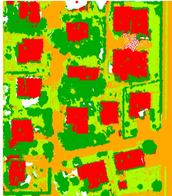
Figure 4. Result of classification in 2D. Legend: Red dots = 'building', brown dots = 'road and parking lot', bright green dots = 'grass', dark green dots = 'tree and hedge'.
