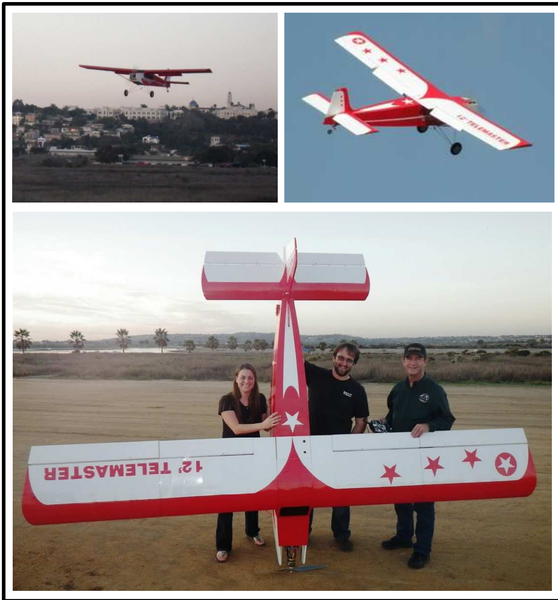
Figure 2. Remotely piloted UAV imaging platform owned and operated by San Diego State University.
