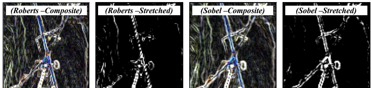
Figure 6. On the left, the Roberts operator is applied to the Road Network Subscene. The Roberts operator clearly depicts the linear features in the scene. Band 140 was histogram stretched in order to optimize edge information along the main linear feature, and modestly improved the interpretability of the feature. Reliable edge information also is visible along several of the smaller roads in the scene as well as along the contours to the west. The mineral deposit to the northeast is clearly recognizable. On the right, the Sobel operator is applied to the Road Network Subscene. The Sobel operator outperformed the Roberts operator, and generated reliable results against the linear features. Band 5 was histogram stretched in order to optimize edge information along the primary manmade linear feature in the scene, which modestly improved interpretability.
