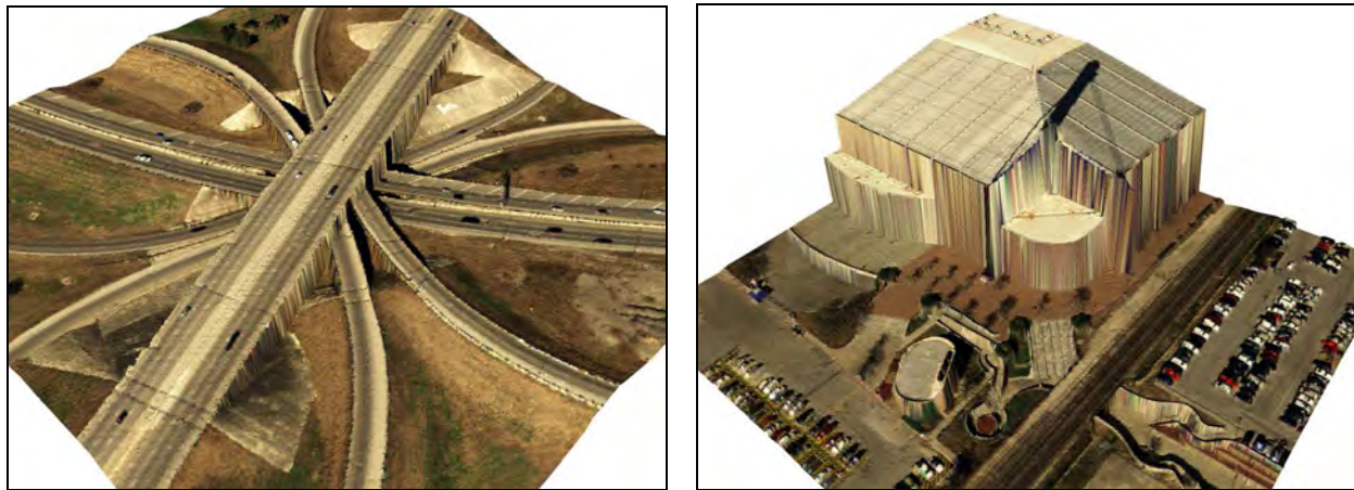
Figure 2. TIN representations of RGB image clouds from San Antonio, Texas; automatically derived from 15 cm ADS imagery without no manual post-processing involved.
