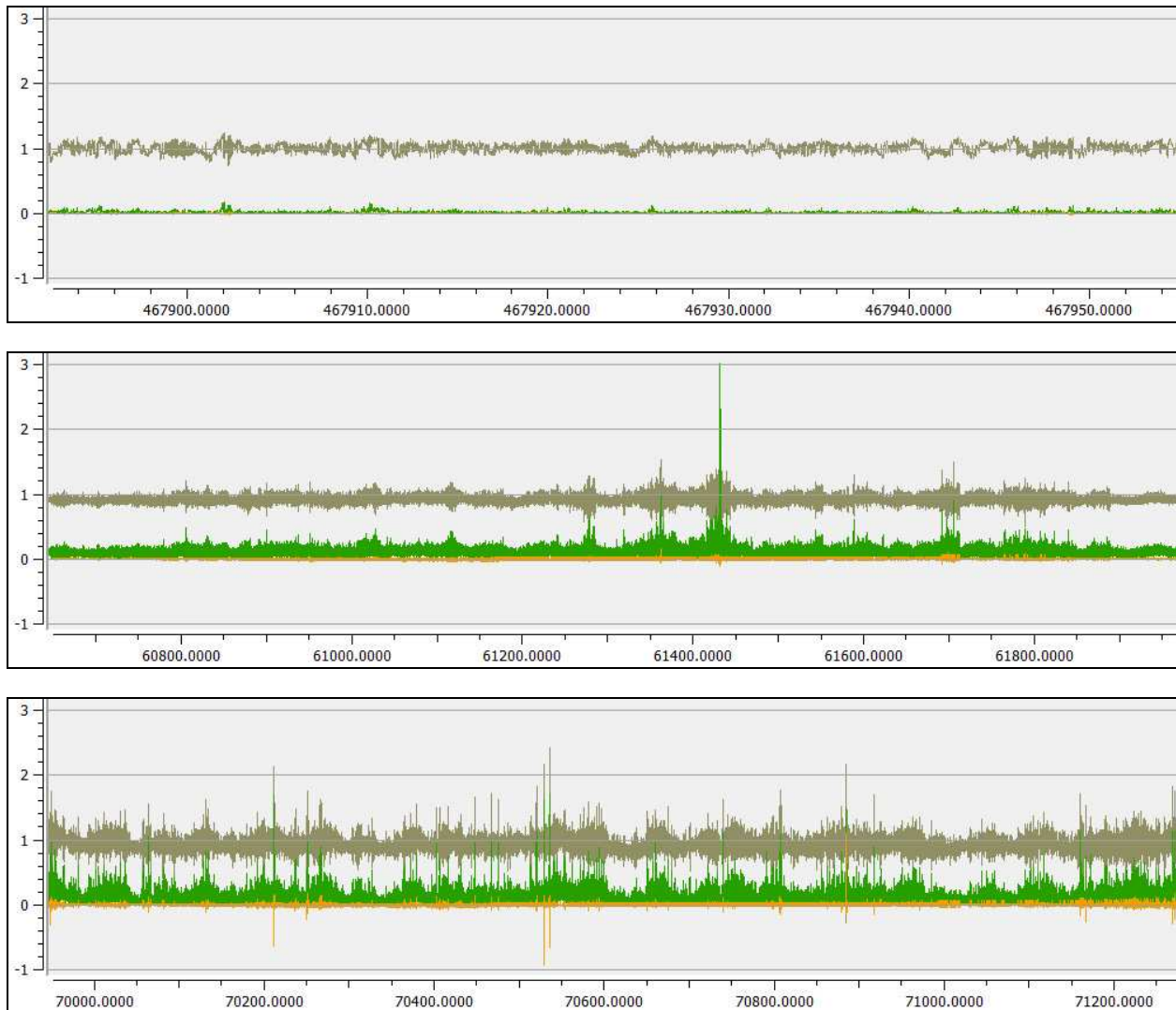
Figure 5. Quality parameter plots for entire ADS takes with different atmospheric turbulence: NCS (grey), PSR (green) and RPE (orange) as functions of GPS time. Top: Romanshorn 10 cm, take 957, with very low turbulence. Middle: San Antonio 15 cm, take 050, with generally little turbulence but one event of smearing ( PSR \sim 3 ). Bottom: San Antonio 15 cm, take 050, with a few cases fast forward coverage ( NCS > 2 ) and backward moves ( NCS < 0 ), corresponding artifacts ( |RPE| > 0 ) and a little bit of smearing ( PSR \sim 1.5 ).
