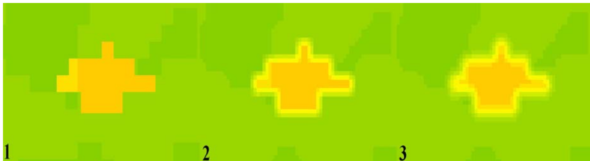
Figure 7. CCM cost surfaces from no smoothing filter (1), filtered with one pass (2), filtered with two passes (3).
