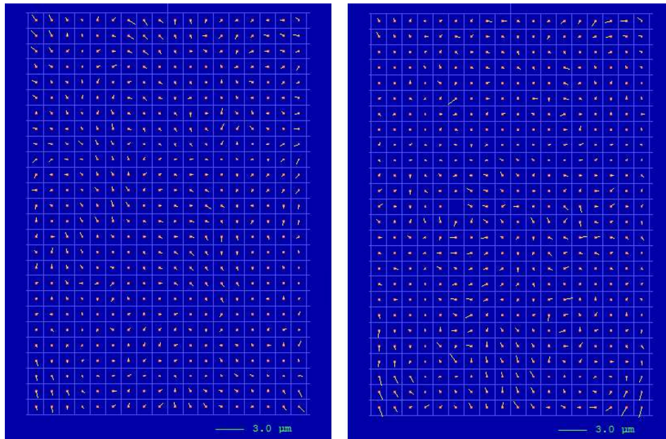
Figure 4. Plot of remaining image residuals for UltraCam Xp (left) and UltraCam L (right). Tiling structures and / or CCD sub areas are not visible.
