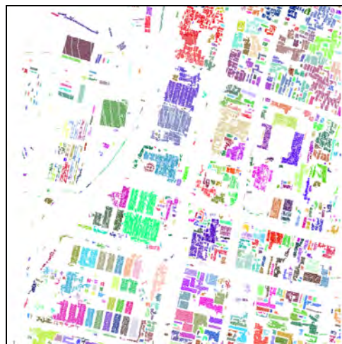
Figure 3. Separated individual building points.
