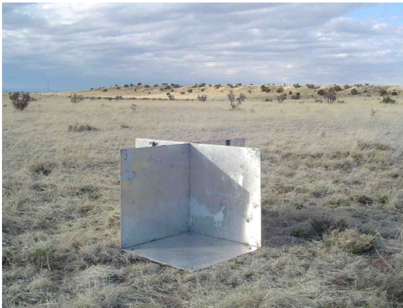
Figure 8. A corner reflector placed in the desert.
