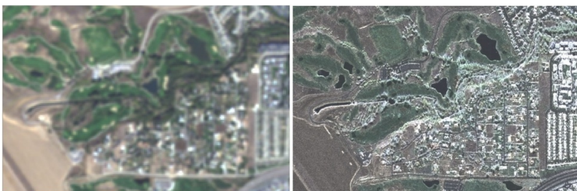
Figure 3. The left image is an ALOS satellite image with 10-meter pixel resolution; the right image shows this same ALOS image “pan-sharpened” with an IFSAR ORI image having 1.25-meter pixel resolution. All features on the right are much clearer, as needed by potential users of orthoimagery in Alaska.
