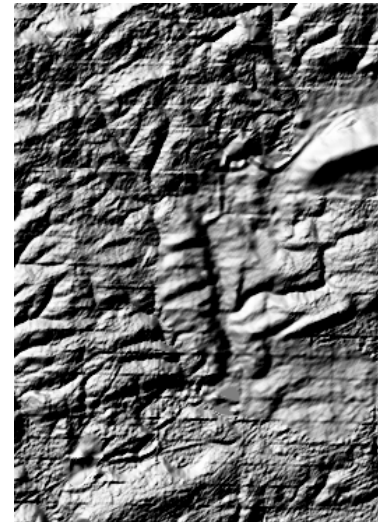
Figure 2. Bad quilting artifacts in quad created with GPM. Visually observed artifact distance = approx. 16 pixels between both horizontal and vertical stripes. Quad name: Bloomsburg, PA. Vertical exaggeration: 5X.
