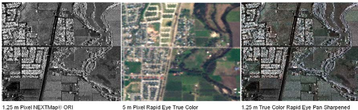
Figure 4. Right Image - Intermap's NEXTMap® Orthorectified radar Image (2 m RMSE horizontal accuracy; 1.25 m pixel); Middle Image – Orthorectified (using NEXTMap® Data) Rapid Eye True Color Image (5 m pixel); Left Image – pan-sharpened Rapid Eye/ NEXTMap®.
