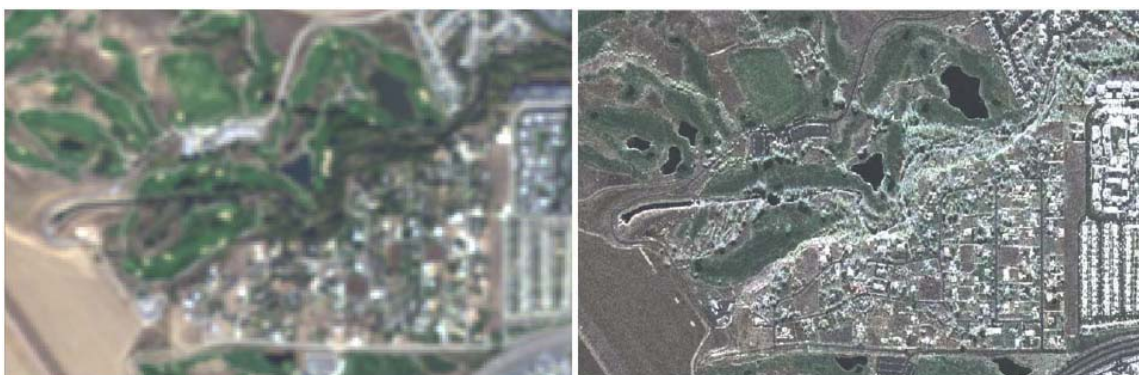
Figure 1. ALOS on left – 10 m pixel resolution (courtesy of ASF) compared with a Pan-sharpened ALOS – Intermap Orthorectified Radar Image on the right (courtesy of Intermap) 1.25 m pixel resolution.
