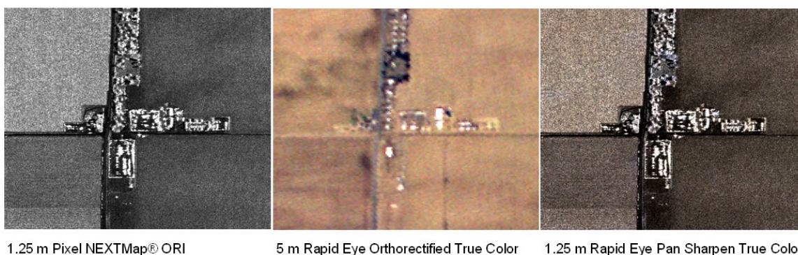
Figure 2. Right Image - Intermap's NEXTMap® Orthorectified radar Image (2 m RMSE horizontal accuracy; 1.25 m pixel); Middle Image – Orthorectified (using NEXTMap® Data) Rapid Eye True Color Image (5 m pixel); Left Image – pan-sharpened Rapid Eye/ NEXTMap® Data.
