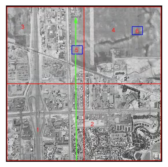
Figure 5: Smaller boxes within the upper-left tile of Figure 4. Their associated densities appear in Table 1 using the boxed area divided by point count method. The differences in densities are functions of position with respect to nadir and local variability of the terrain. Areas with vegetation and multiple returns increase density or bias the statistic. The nadir position is shown as a green line passing through area 5.
