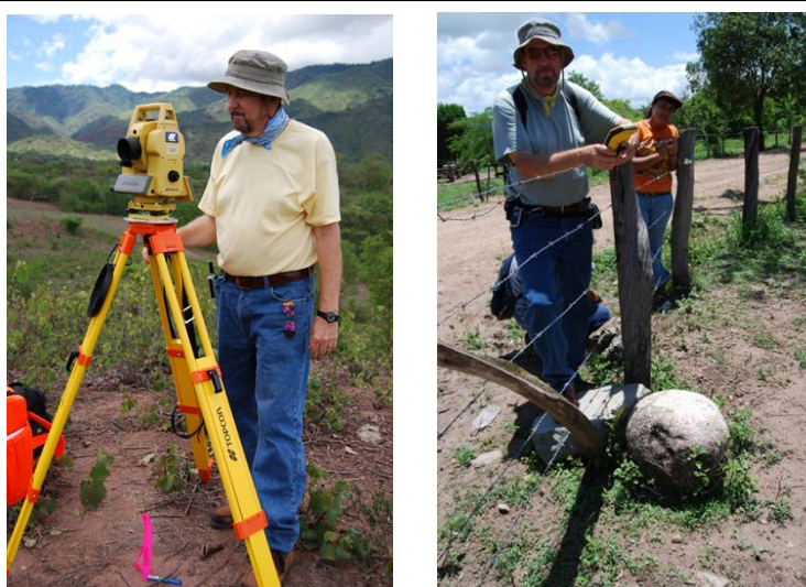
Figure 5. Mapping with laser total station, (left). Recording artifact positions with GPS data collector, (right).
