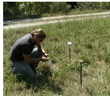
Figure 3. Deploying model penetrometers.
