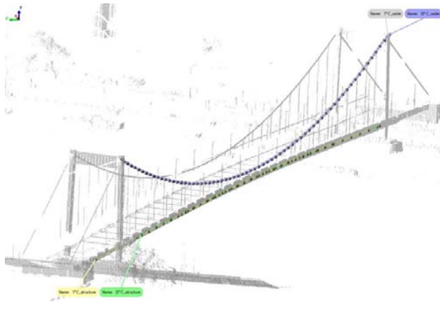
Figure 11. Modeling the main cable and the deck.
