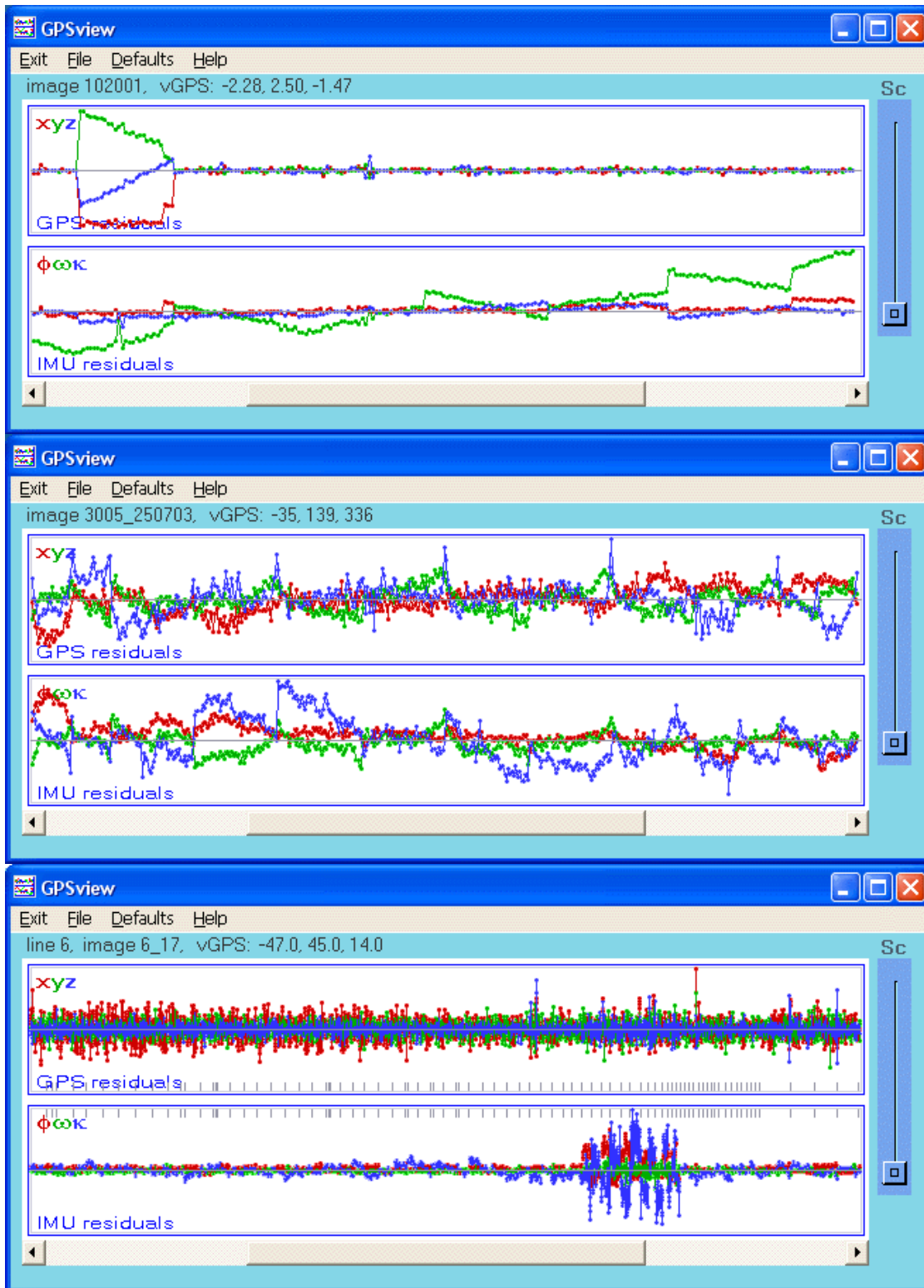
Figure 9. GPS/IMU residuals from different projects. Systematic effects and relations between GPS and IMU data can be easily identified.
