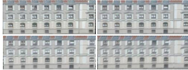
Figure 6. Of one single façade of one building will obtain multiple aerial image segments. These have been rectified into a façade coordinate system. From an aerial image block showing for each object point typically 10 images, not all will contain useful data for a specific vertical façade. Selected here are the 4 best, where “best” is defined as the largest area of a façade quadrilateral in the projection into an image.
