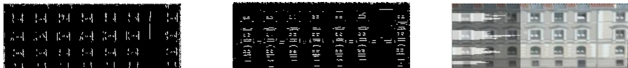
Figure 7. Binary Prewitt edges in (a) are vertical, in (b) horizontal. The sums of edge values are shown in (c) as a count of the number of floors.
