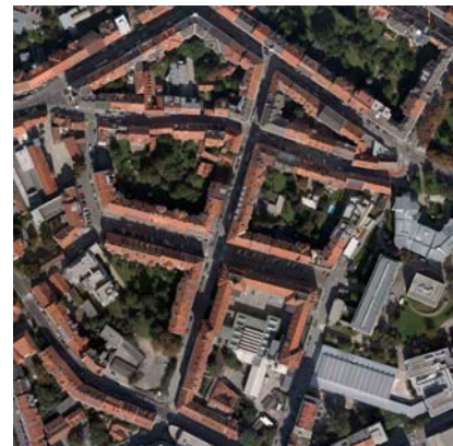
Figure 3. A 400 m x 400 m segment of an orthophoto of the urban core of the city of Graz (Austria). The pixel size is at 10 cm. The orthophoto is of the type “true”; therefore the facades are not visible.
