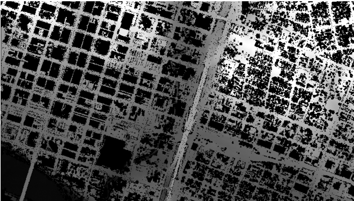
Figure 10. Ground filtering results from the interpolated first return image. White stands for ground feature rendered in elevation and black represents non-ground features.
