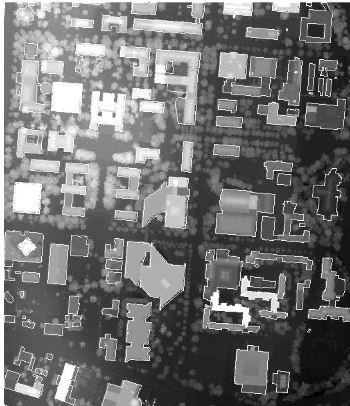
Figure 7. The lidar first return and building ground truth data overlay (size is changed for displaying purpose) (Meng, Wang, and Currit, 2009).
