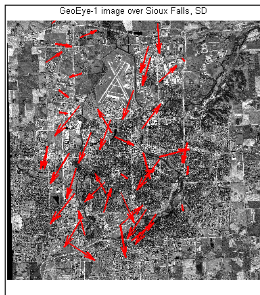
Figure 3. Error plots from the I2I analysis of GeoEye-1 imagery over Sioux Falls.
