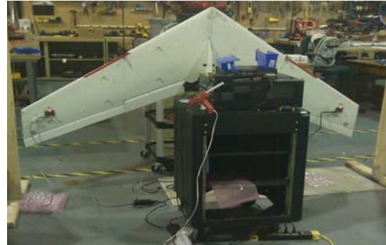
Figure 6. Front view of experimental setup with cameras mounted at wing tips.
