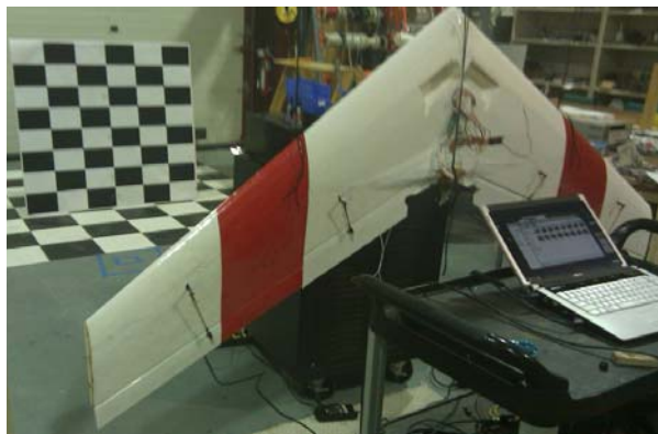
Figure 7. Reverse view of experimental setup with calibration target in view. Additional objects were placed in front of the system for distance measurements during the experiment.
