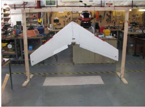
Figure 5. Experimental flying wing suspended from wooden frame with bungee cords.
