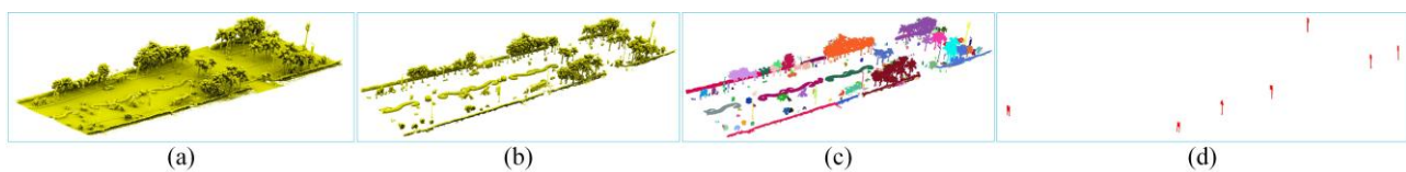
Figure 1. (a) A raw point cloud, (b) off-ground points after ground removal, (c) clustered off-ground objects, and (d) detected 3D traffic signposts.
