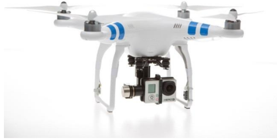
Figure 2. The small DJI Phantom 2 UAV drone with GoPro camera mounted
