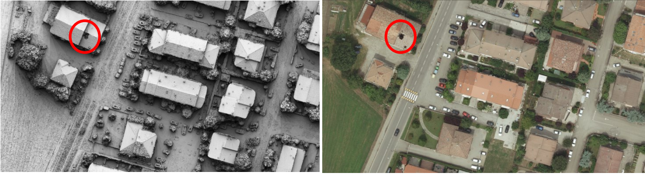
Figure 1: Generated point cloud in shaded view (a) and corresponding true ortho-photo automatically generated (b): little collapsed parts of the building are visible both from 3D and 2D data (red circles).
