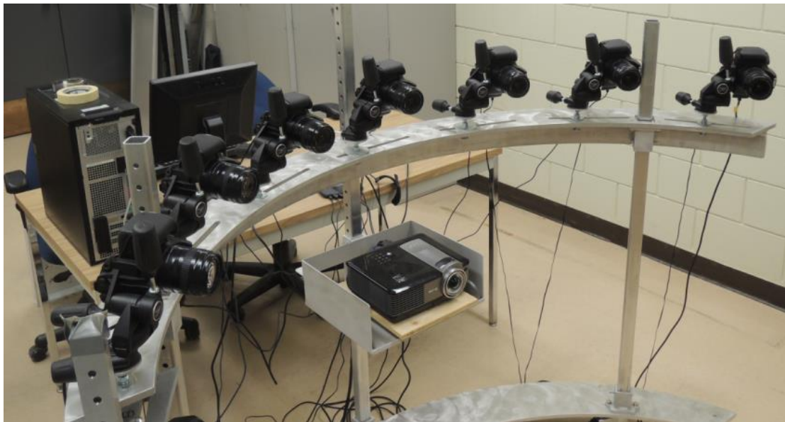
Figure 2: A close-range multi-camera photogrammetric system
