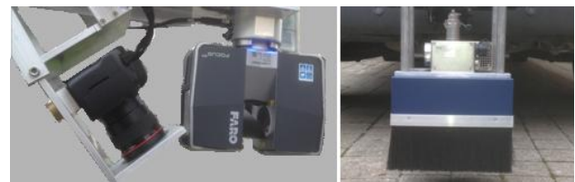
Figure 2. Canon camera, FARO laser scanner and Polytec spectrometer head
